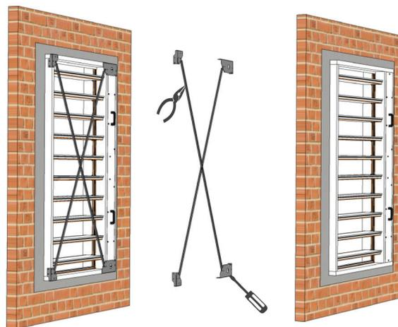
After installing the damper and the gypsum/Firebatt has hardened, the supports of the damper, transport struts and corners can be removed.
