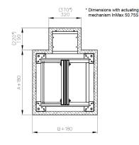
Insertion depth typically 250 mm for dampers supplied with flanges, and 200 mm for dampers without.
