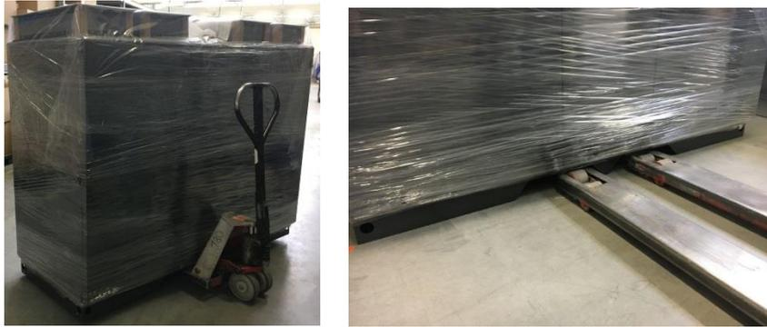
Openings are provided in the frame of the units for handling. During use, pallet truck forks must remain fully under the chamber.
