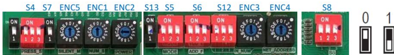
Fig. 29: Micro switches on the main board of the outdoor unit
