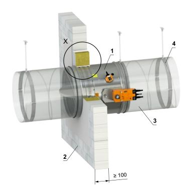
\*\* For fire resistance EI 45 S is approved opening between the construction and the damper in the range of 30...75 mm.
