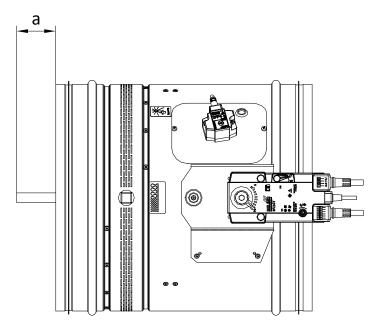
Values "a" has to be respected when projecting following air-conditioning duct.
