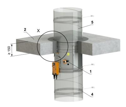
\* For fire resistance EI 45 S is approved opening between the construction and the damper in the range of 50...150 mm.
