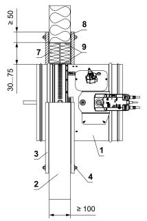
\* HILTI system can be replaced by a similar system with the same or higher thickness, density, fire reaction class, tested according to EN 1366-3.
