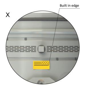
"BUILT IN EDGE label" indicates the recommended edge of installation of a fire damper in the fire separating construction (wall/ceiling). The damper must be installed so that the entire damper blade (in the closed position) is located in the fire separating construction (wall/ceiling) and at the same time the actuating mechanism and inspection openings are freely accessible.
