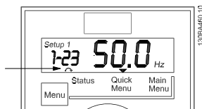
Illustration 7.7 Indicating Motor Direction
