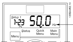
Illustration 7.6 Indicating Unit of Selected Parameter
