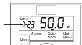
Illustration 7.4 Indicating Selected Parameter Number
