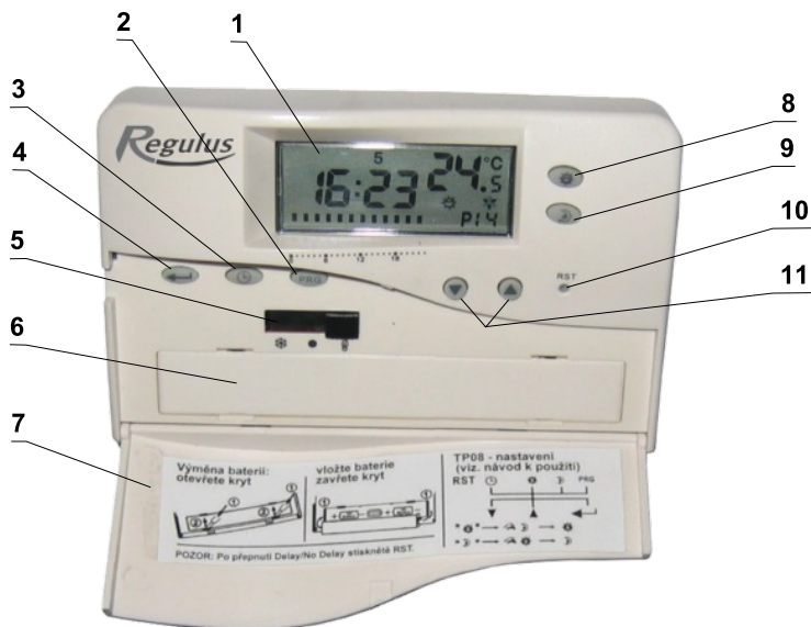
Fig.3 Programmable room thermostat TP08
