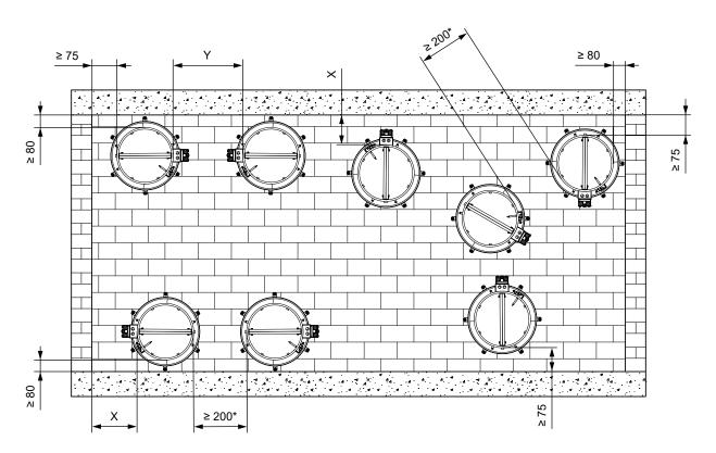
X = recommended min. distance ≥ 220 mm required to access the actuator or manual control
