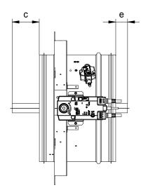
Blade overlaps of FDMS with VAV actuator
